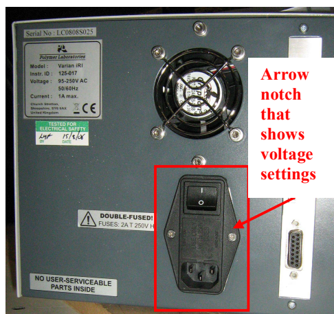
Figure 4: Back Panel of the RI Detector
